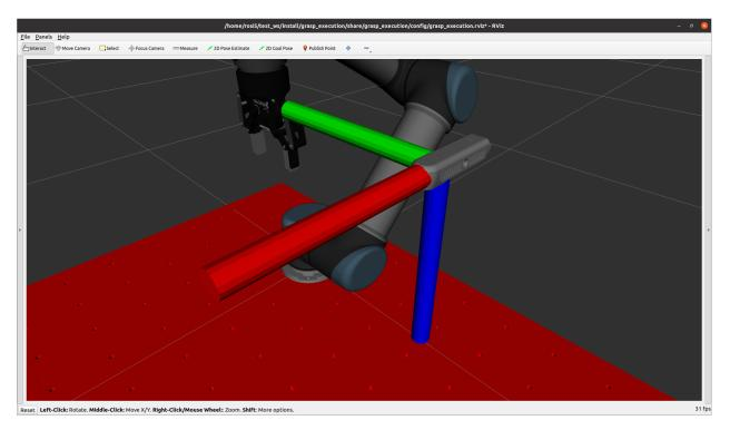
To do so, we need to add a link in this orientation in the URDF. In the file /workcell\_ws/src/scenes/new\_scene/ urdf/scene.urdf.xacro add the following lines under the declaration of the camera object:
