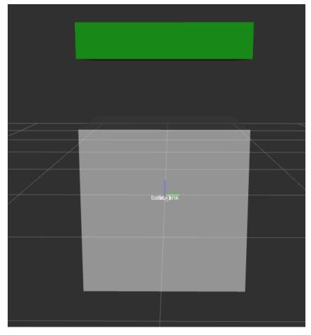
This configuration shows a link connected to the base\_link with a joint origin of 0,0,0 and the visual mesh of link has an origin of 0,0,1. As you can see, link's tf is at the 0,0,0 of base\_link, while the visual component of link is at 0,0,1 from the tf of link
