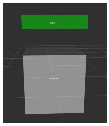
In this configuration however, shows a joint origin of 0, 0, 1 and the visual mesh of link has an origin of 0, 0, 0. As you can see, link's **tf** is at the 0, 0, 1 of base\_link, while the **visual** component of link is at 0, 0, 0 from the **tf** of link
