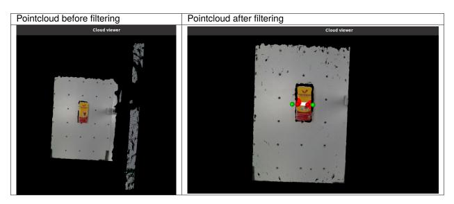
As shown above, unnecessary information on the right side of the pointcloud was removed. Limits can be set even tighter in order to crop out more of the work surface.
